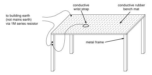
Figure 1.1 Typical Antistatic Bench Set Up
